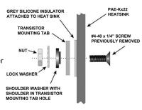
Your Kx22 Heatsink should have come with the thermal pads, foam block and copper tape pre-mounted on it.
