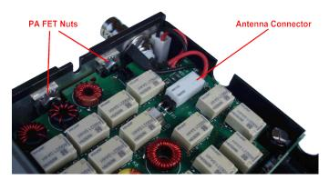
Locate the two #4-40 screws which hold the PA-FETs to the Elecraft end panel. The captive lockwasher #4-40 nuts should be held with needle-nose pliers while the screws are removed.
