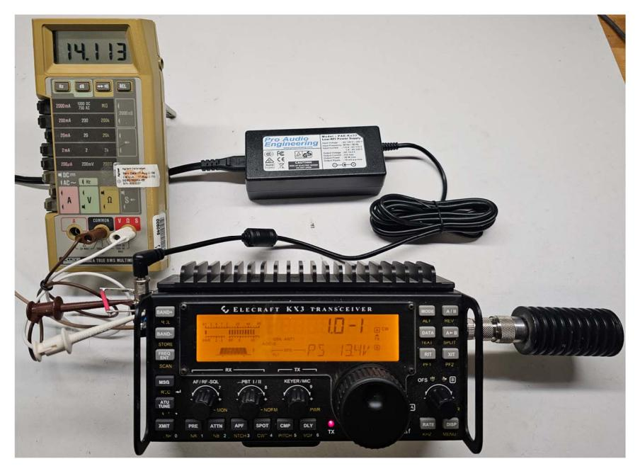
The Kx33 supply is delivering 14.113 V to the KX3 DC input jack, and the KX3's internal voltage displayed is 13.4 V, which is 713 mV less.
