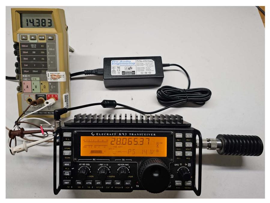
The PAE Kx33 supply is delivering 14.383 V to the KX3 DC power jack, so it has dropped by only 0.025 V at 195 mA output current. This is entirely due to the small resistance of the Kx33 DC output cable and the resistance of the Kx33 plug to the measuring fixture jack. The Kx3 shows the DC voltage as 14.1 V, so it's indicated voltage is 0.283 V lower than the actual input voltage when in receive at 195 mA current draw.
