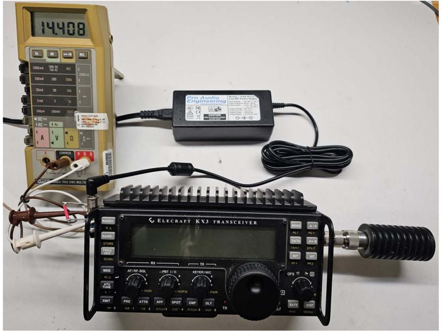
We then turned on the KX3, so this picture shows the DC voltage at the DC input jack with the KX3 drawing an indicated 0.195 A (195 mA):
