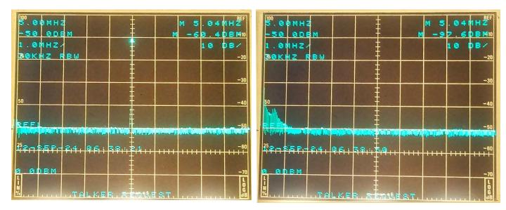
Although we guarantee less than 10 mV peak to peak from 1.8 to 30 MHz, the actual average RF output is much lower, for this particular Kx33 around 1.5 mV RMS, and that energy is concentrated below 1 MHz as the sweep shows. From 1.3 MHz to 10 MHz (sweep limit) the energy is at the noise floor of the Tektronix 2712 spectrum analyzer. These supplies do not output RF on the DC cable!
