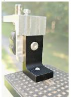
The AM1-TA (shown with a silver AM1 for clarity) adapts the AM1 bracket for tripod mounting on any standard camera tripod which has a 1/4-20 threaded stud mount. Machined from billet 6061 aluminum, it is a full 1/4" thick for rigidity and full thread engagment for both the AM1 knurled bolt and tripod threaded stud.
