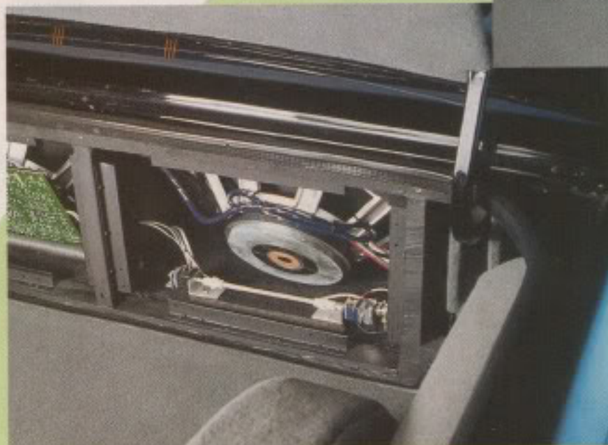
Below the woofer are volume servos that automatically adjust the gain at various points in the signal chain.
