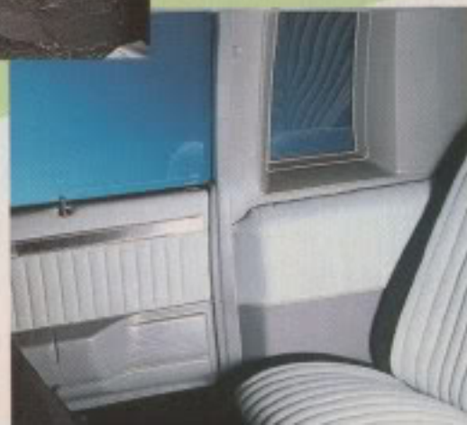
Below: Absorption material was added to almost all upholstered interior surfaces.
