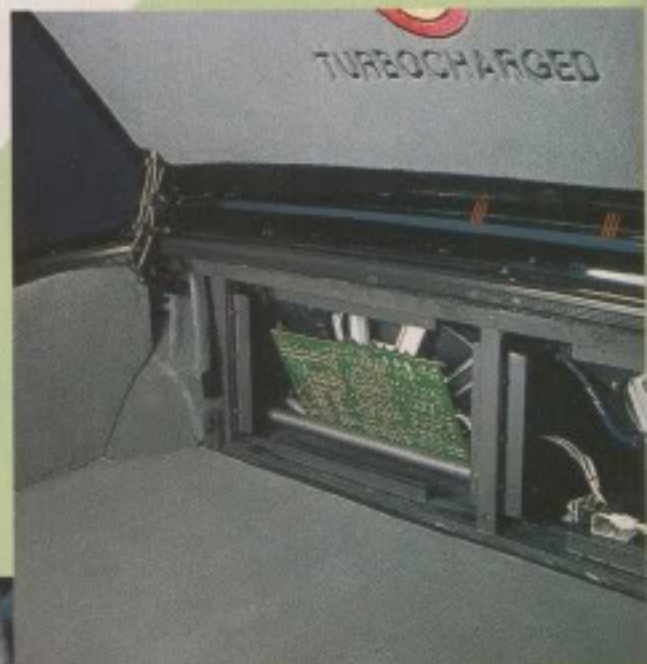
Right: Signal processor and servo controller in aperiodic subwoofer enclosure.
