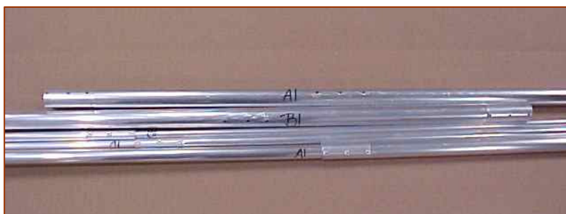
“A” and “B” MARKINGS ON ELEMENT PIECES “A1” & “B1” identify they are part of element #1.
