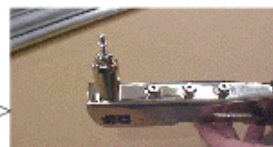
6) Mandrel removed from rivet tool
