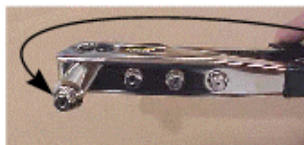
RIVET TOOL NOZZLE <--Wrong one on left - hole is too large Correct on right - small hole fits mandrel --> (rivet shown dropping into nozzle)
