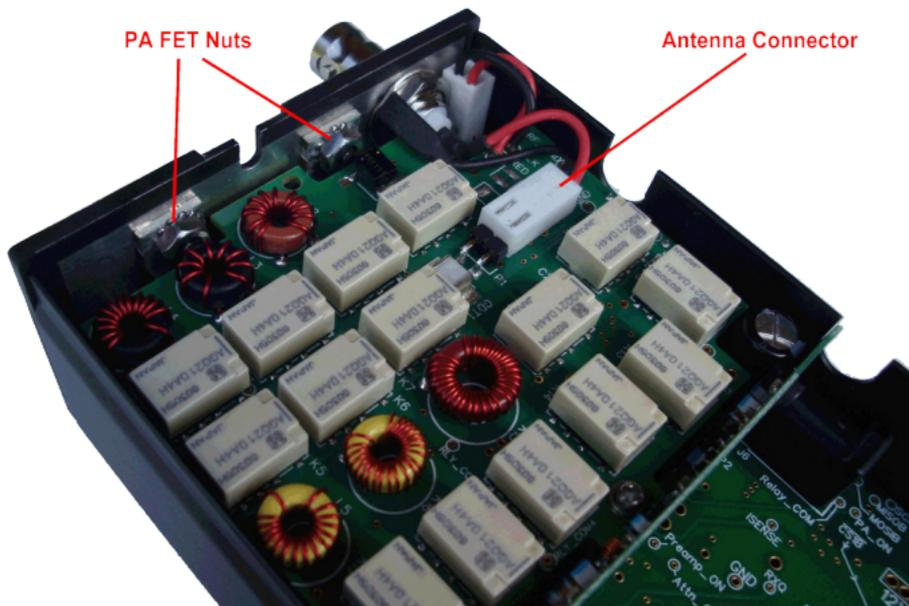
Unplug the antenna connector from the main PCB or from the KXAT2 board if so equipped.
