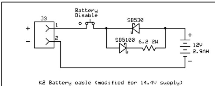
The necessary components to perform the modification are available from PAE in the #33-225 K2 Charger Mod Kit. The additional SB5100 Schottky diode drops the charge voltage by 0.4-0.5V depending on the state of charge of the battery. This will result in charge characteristics similar or better than stock.
