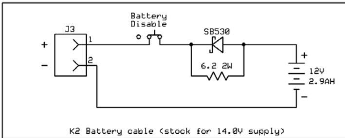
The circuit is designed to operate from 14.0V +/- 0.2V. The SB530 Schottky diode allows for full battery discharge current and voltage minus the 0.2V drop across the diode, while the 6.2Ω 2W resistor limits charge current. When the battery is fully charged it draws ~15-30mA, so in float charge there will be a ~0.1-0.2V drop over the 6.2Ω resistor.
